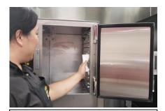
Replace steam collector and pan rail. Wipe all surfaces inside the steamer with a dry wiper towel.
