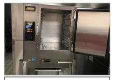
The steamer door is kept open when steamer is off to allow moisture to escape.
