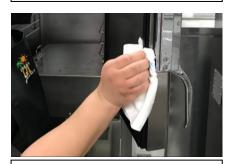
Wipe the rubber gasket around the door with a dry wiper towel to remove all moisture.
