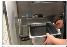
Place hotel pan at the bottom of steamer to avoid spills when the release valve is opened.
